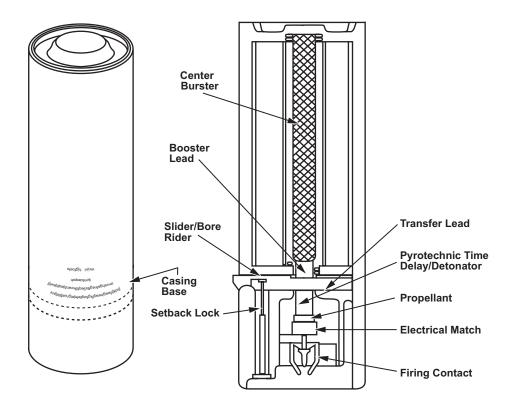
Figure D-10. M82 Smoke Grenade.
