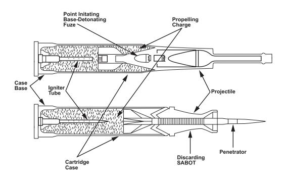
Figure D-1. Example of 120mm Main Gun Ammunition Markings.
