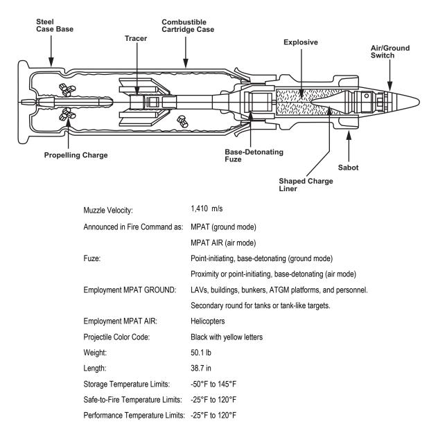
Figure D-5. M830A1 HEAT-MP-T (120mm).
