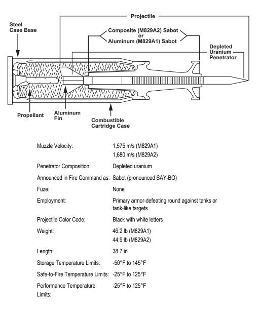
Figure D-2. M829A1/M829A2 APFSDS-T (120mm).
