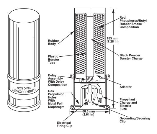
Figure D-8. L8A1 and L8A3 Smoke Grenade.
