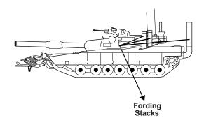
Figure 7-1. M1A1 Tank with Fording Kit.
