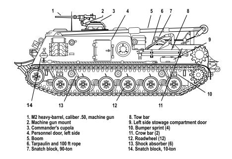
Figure A-2. M88A2 Recovery Vehicle.
